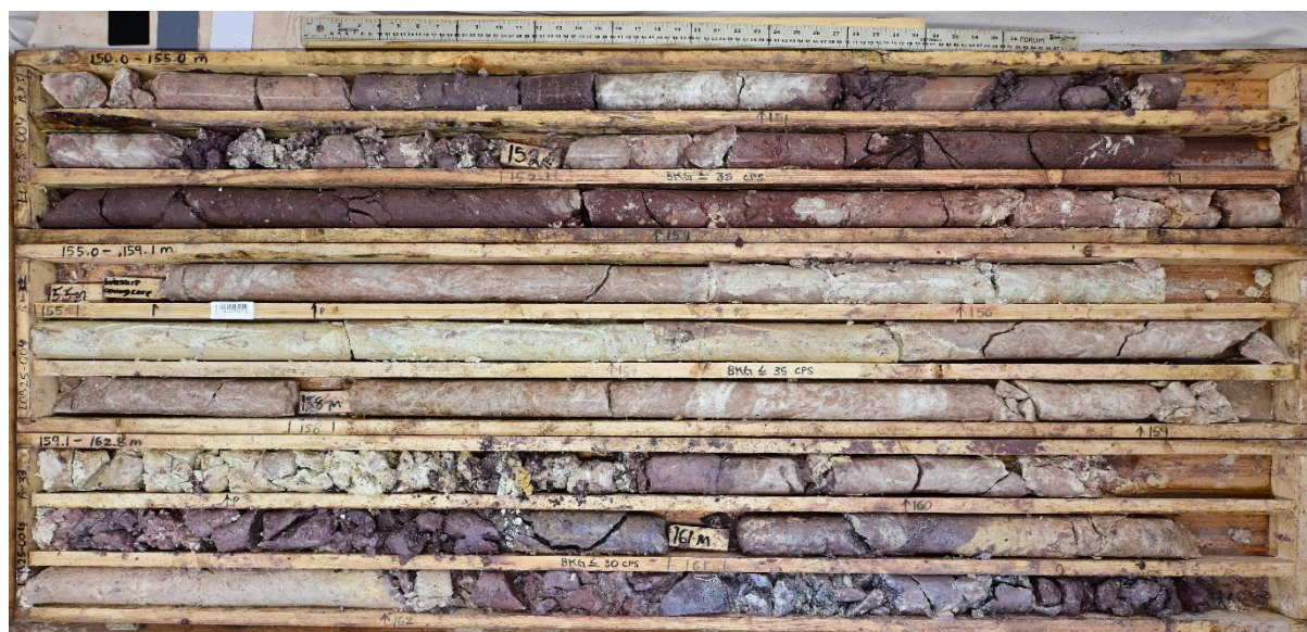
Figure 11: Drill core from LOB25-004 showing pervasive strong clay alteration, patchy bleaching and remobilized specular and red hematite. The core is completely replaced by clay and overprints earlier silicification.
