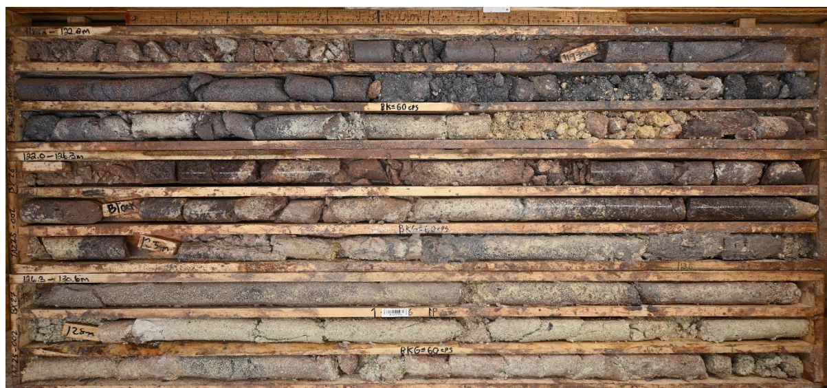
Figure 9: Drill core from TAZ24-002 showing pervasive strong clay alteration, patchy bleaching and remobilized specular hematite. The core is completely replaced by clay.
