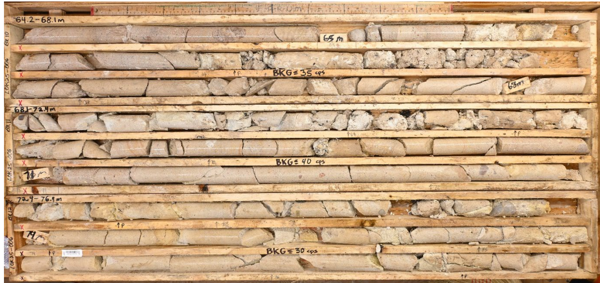
Figure 4: Drill core from LOK25-006 showing pervasive strong clay alteration and bleaching as well as numerous post Thelon Basin faults.
